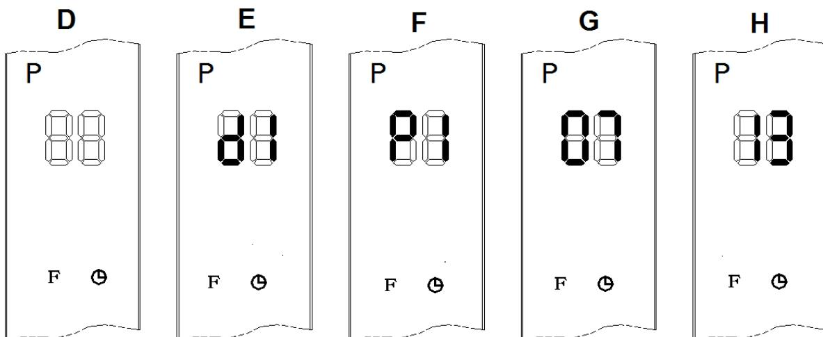
8. Press the plus and minus buttons to set the required temperature.
